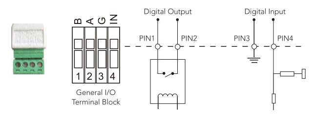
PIN1: Alarm Output NC / NO 24V DC 1A PIN2: Alarm Output NC / NO 24V DC 1A PIN3: Alarm Input NC / NO ≤12V PIN4: Alarm Input NC / NO ≤12V
